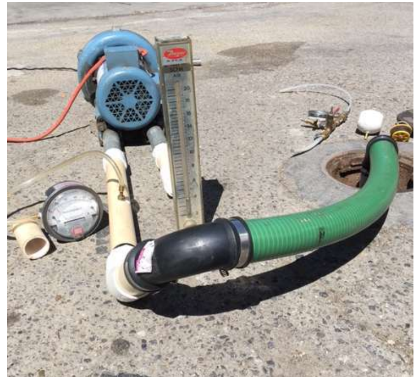
1-hp blower powered by a residential (15A) outlet (up to 60 scfm)
