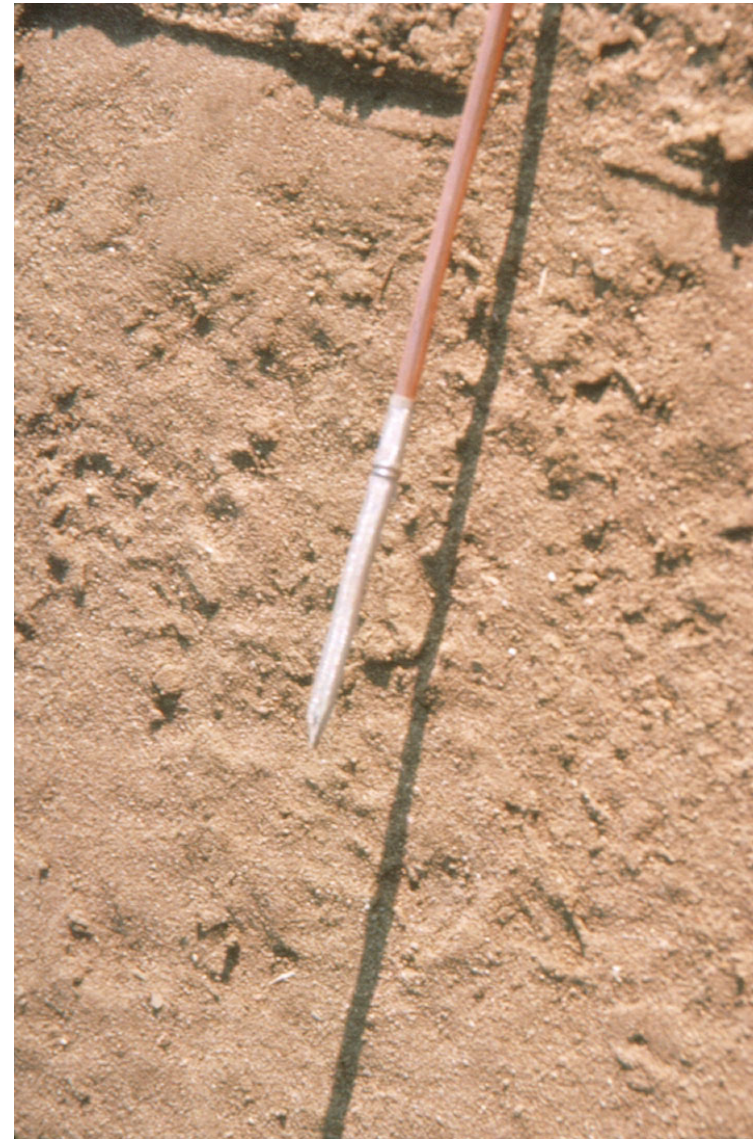
Examples of probes used to monitor pressure and sample soil gas at Traverse City, MI.
